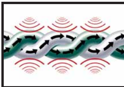
Illustration 2: Example of Bonded Pair. As cable is stretched and pulled, pairs stay intact.
